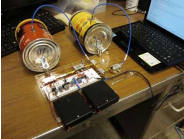
Innovation: Plexiglas radar chassis for improved ruggedness for use in field testing
