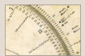
Created in 1843, Palmer's is reputed to be the first computing scale produced in America. It consisted of logarithmic combinations of numbers, arranged on two circles, one revolving within the other, and was intended to solve the most difficult mathematical problems. It sold poorly, however-in part because of Americans' fear that reliance on such a device would weaken the mind.
