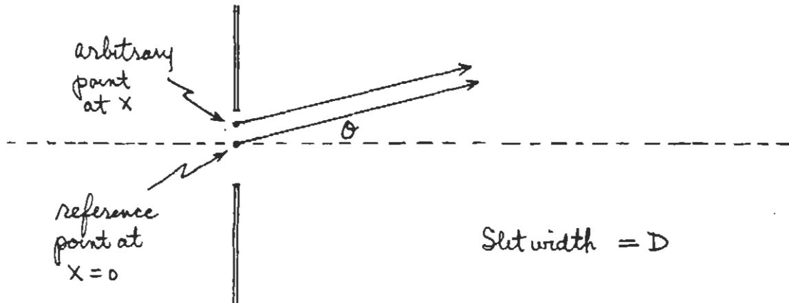
By the same geometry as used for the case of the narrow slits, we find that the relative phase of the radiation emanating from a point  $x$  within the aperture is
