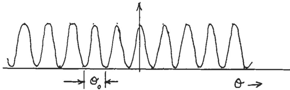
The separation between minima is obtained by allowing the argument of  $\cos^2\left(\frac{\pi \theta D}{\lambda}\right)$  to advance by  $\pi$
