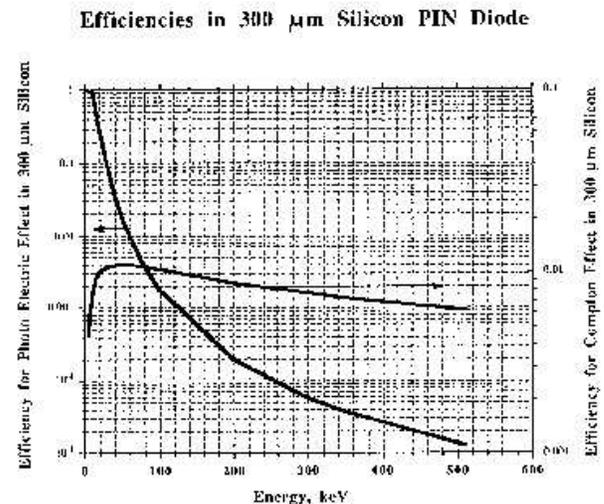
FIG. 3. Photon detection efficiencies in silicon. Note that the vertical axis is logarithmic.
