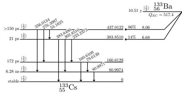
FIG. 5. Decay of  $^{133}\text{Ba}$  to  $^{133}\text{Cs}$  with associated energy levels. The time on the left is the half-life of the state, next to it is the state's spin, and on the right is the energy in keV. The arrows denote the transitions between energy levels in  $^{133}\text{Cs}$ , with energies in keV. Data taken from the Table of Radioactive Isotopes.
