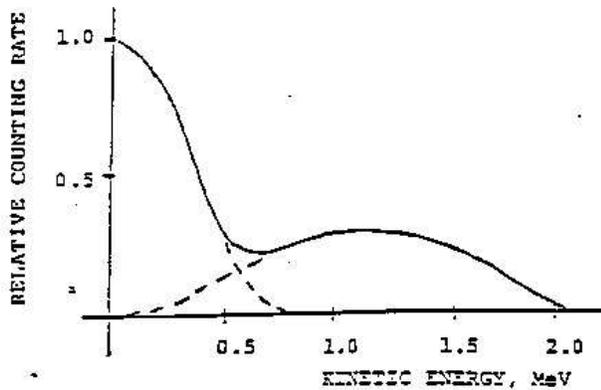
FIG. 2. The  $\beta$ -ray Spectra of  $^{90}\text{Sr}$  and  $^{90}\text{Y}$ . The actual energy spectrum of the electrons in this experiment will be distorted by energy loss of the electrons in the material of the source and in the thin metal covering over the source.
