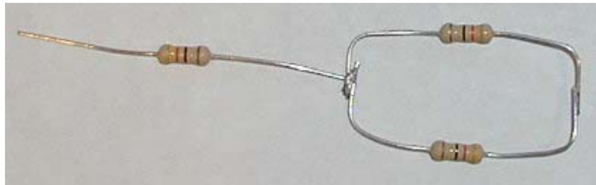
Figure 1: Three 43\Omega Resistors, one in series with two in parallel
