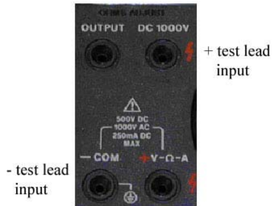
Figure 15: Test lead inputs to multimeter for 1 K range
