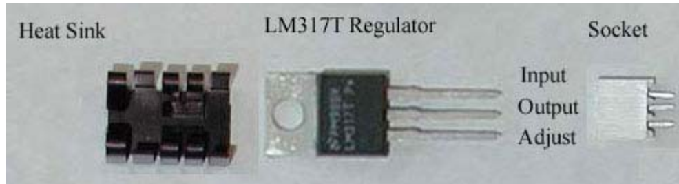
Figure 12: Heat sink, LM317T voltage regulator, and socket
