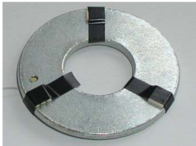
Figure 2: perf-board used as spacers on washer
