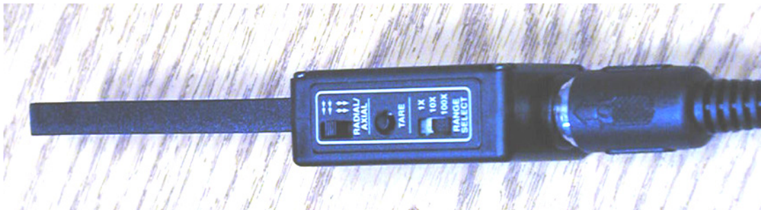
Figure 5 The top of the magnetic field sensor, showing (from right to left) the RANGE SELECT switch, the TARE button, and the RADIAL/AXIAL switch, which is set to RADIAL
