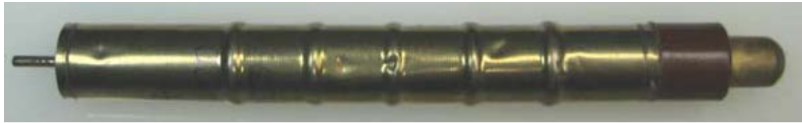
An SBM-20U tube, showing the wire anode
