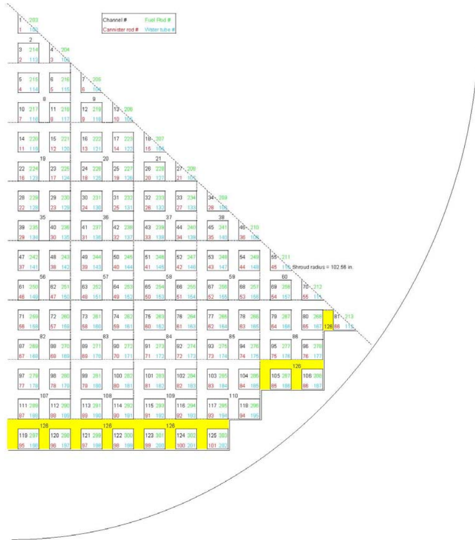
Figure PS2-2: VIPRE Modeling of the BWR/5 Core and Internals
