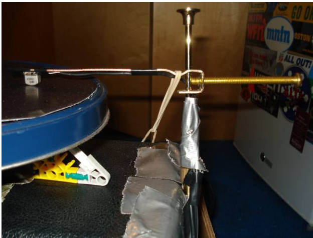
Figure 2: The tape head arm configuration. The arm consists of an appendage to support the tape head on the left and a handle with which to play the TSW on the right
