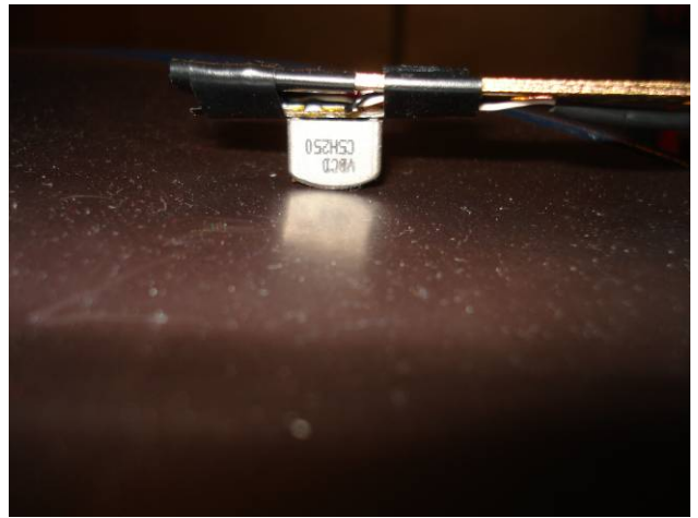
Figure 3: Close-up of the magnetic tape head.
