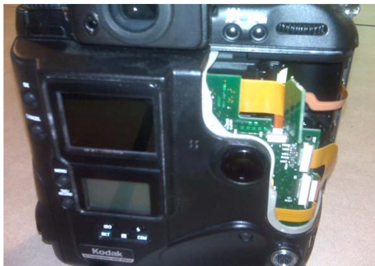
Fig. 1. A primitive NIKON digital camera retaining the traditional form factor of the earlier film cameras. This digital camera even has a space for film inside.
