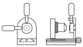
Figure 1: Sketch of a Lens-Pinhole Spatial Filter (LPSF or "beam cleaner")
