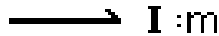
Figure 4.6: Bond graph symbol for an ideal linear kinetic energy storage element with inertance m .
