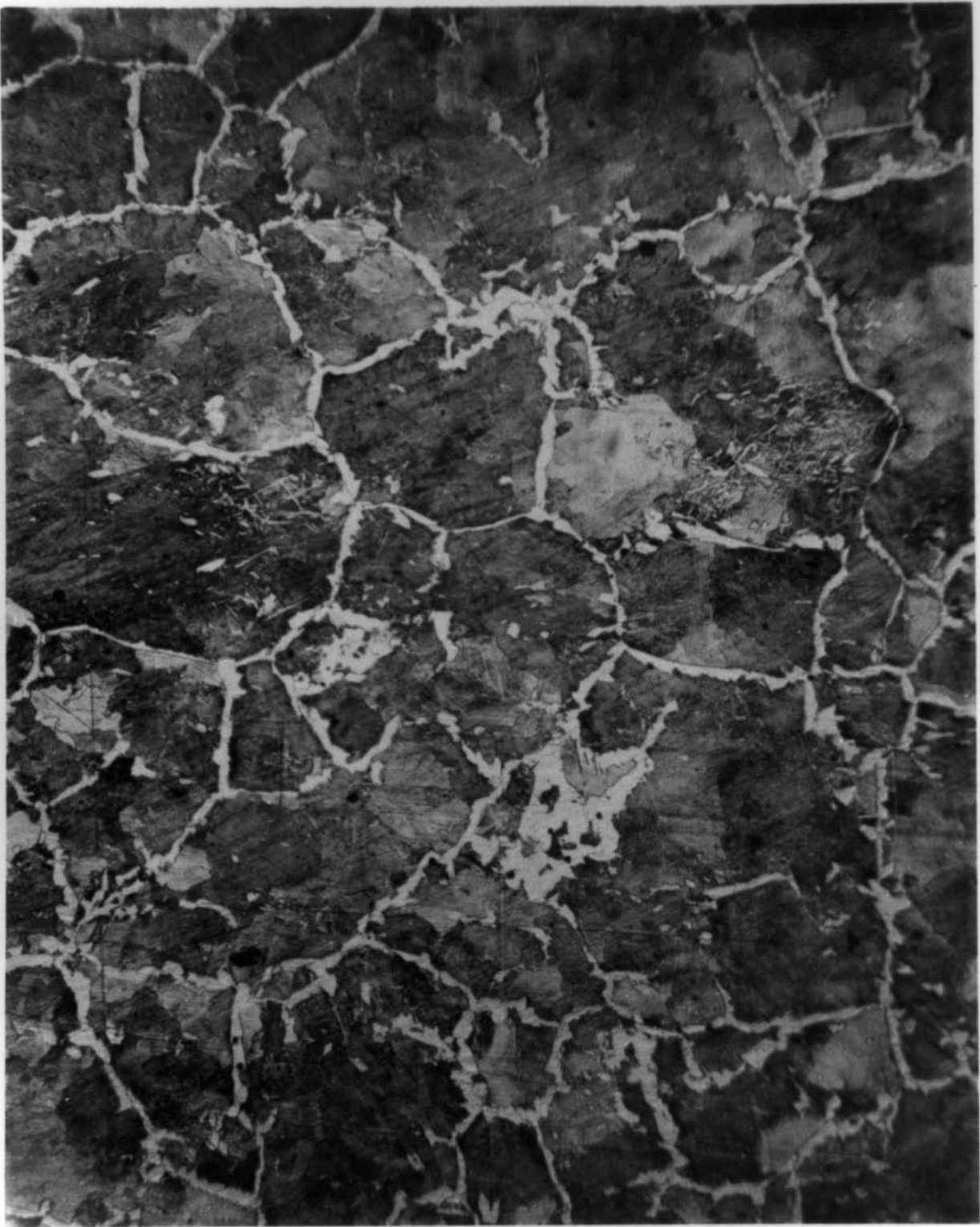
Figure 5: Microstructure of whole bolt. (100X)
