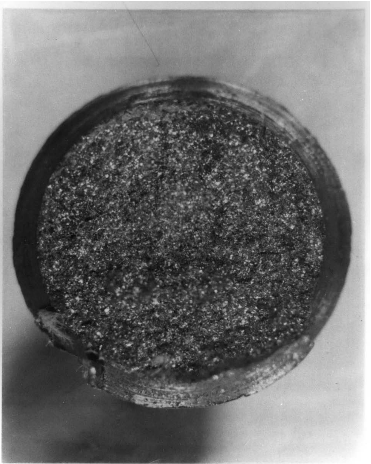
Figure 6: Overall view of fracture surface of failed bolt.
