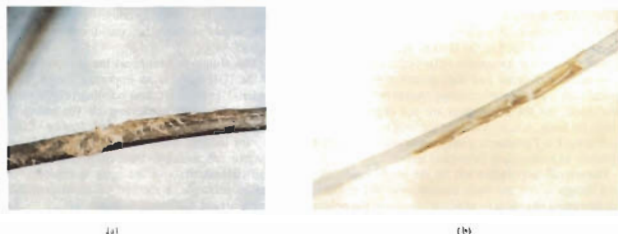
Figure 11. Optical micrographs of used Cu-7 with black polypropylene string (a) and used "T" with blue polyethylene string (b), showing debris encrustation.
