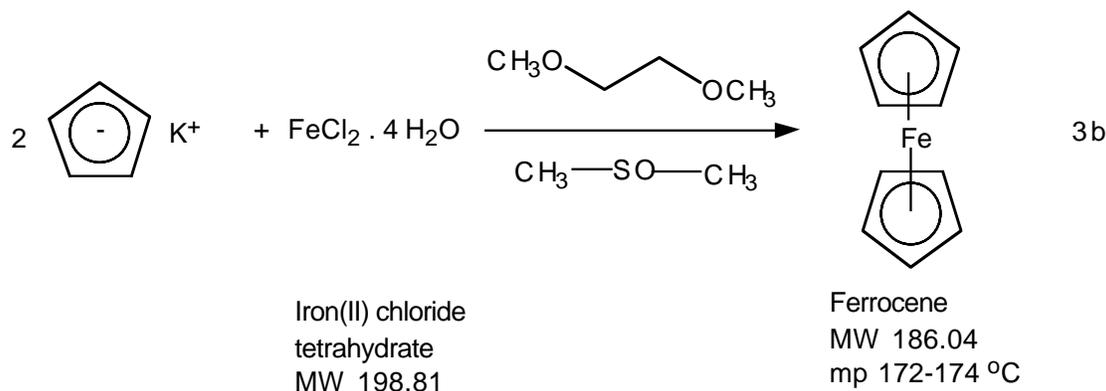
**Iron (II) chloride solution:** Add 0.35 g of finely powdered green iron (II) chloride tetrahydrate\* and 1.5 mL of dimethyl sulfoxide\* to a 4 mL Assem Vial with septum (provided by TA). Cap the flask with the septum provided, insert an empty syringe needle through the septum and then insert the nitrogen inlet needle. Pass nitrogen into the vial for about 1 min to displace the oxygen present. Remove the needles. Shake the vial vigorously to dissolve the iron chloride.
