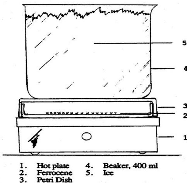
Figure 2: Apparatus for the Sublimation of Ferrocene
