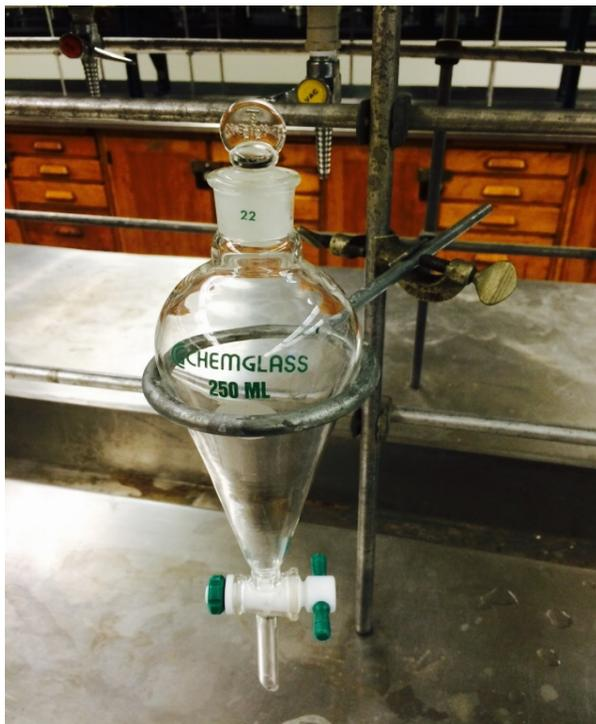
**Figure 5-4 Separatory Funnel with Ring Stand Support**
