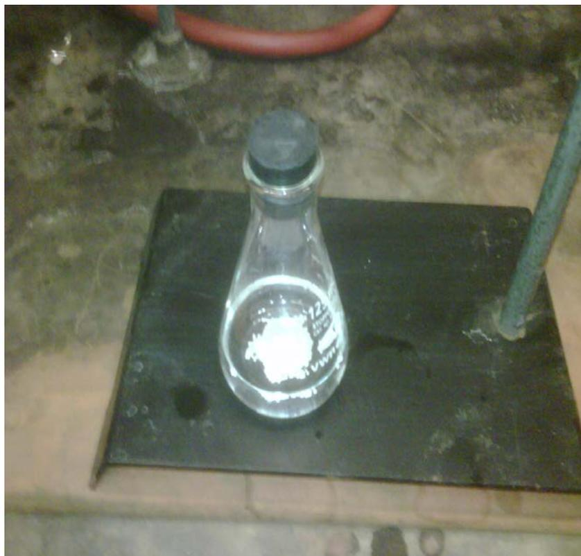
**Figure 5-5** Drying Sample with an Anhydrous Drying Agent
