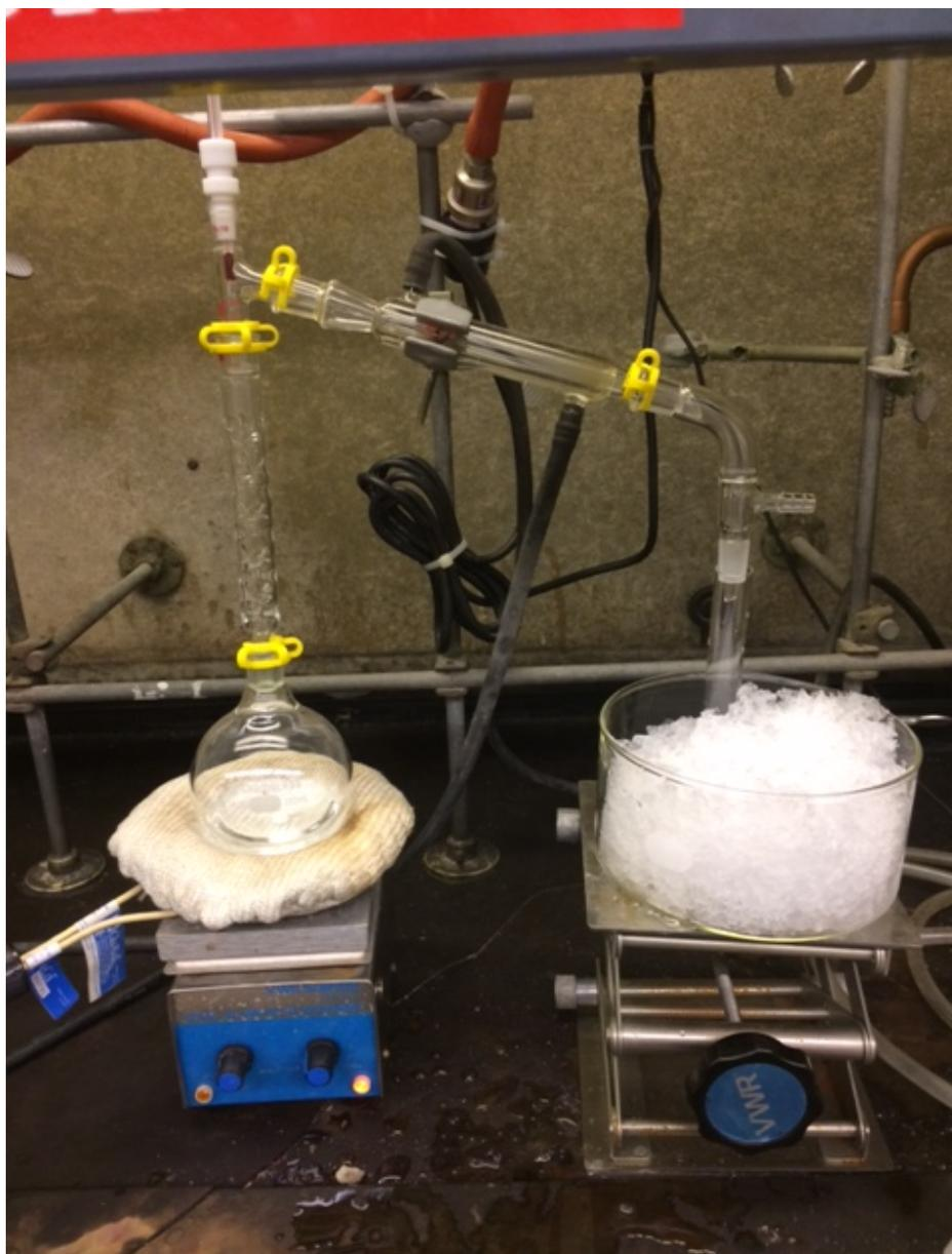
**Figure 5-6 Atmospheric Distillation Apparatus with Vigreux Column**
