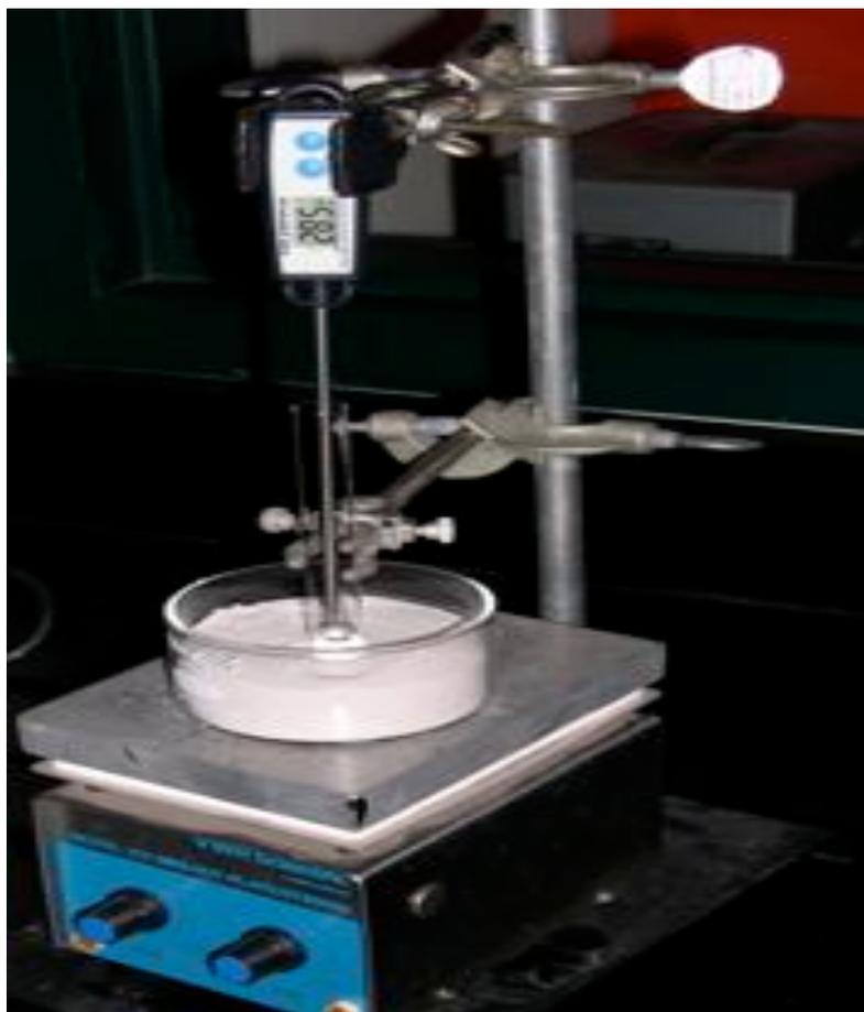
**FIGURE 5-8a** Photo of Boiling Point Apparatus
