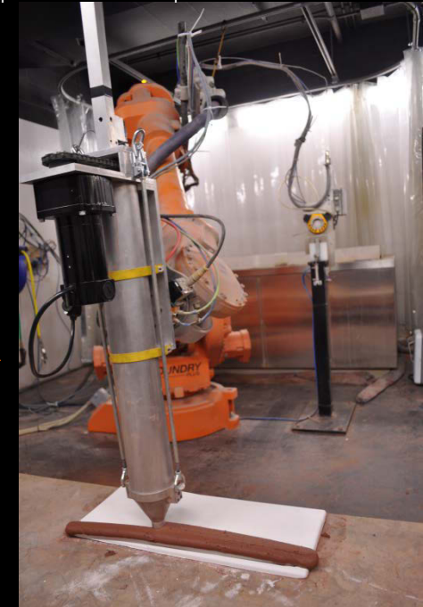
Phase 2 – Building a prototype using the robotic arm with a custom-made extruder controlled by Rhino
