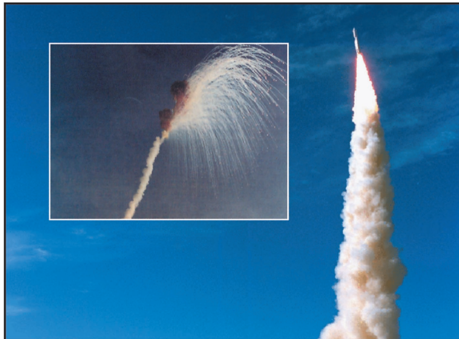
The explosion of a Titan IVA in August 1999 was caused by wiring defects. Titan IV quality problems were linked to the overemphasis on cost-cutting and the loss of experienced personnel.
