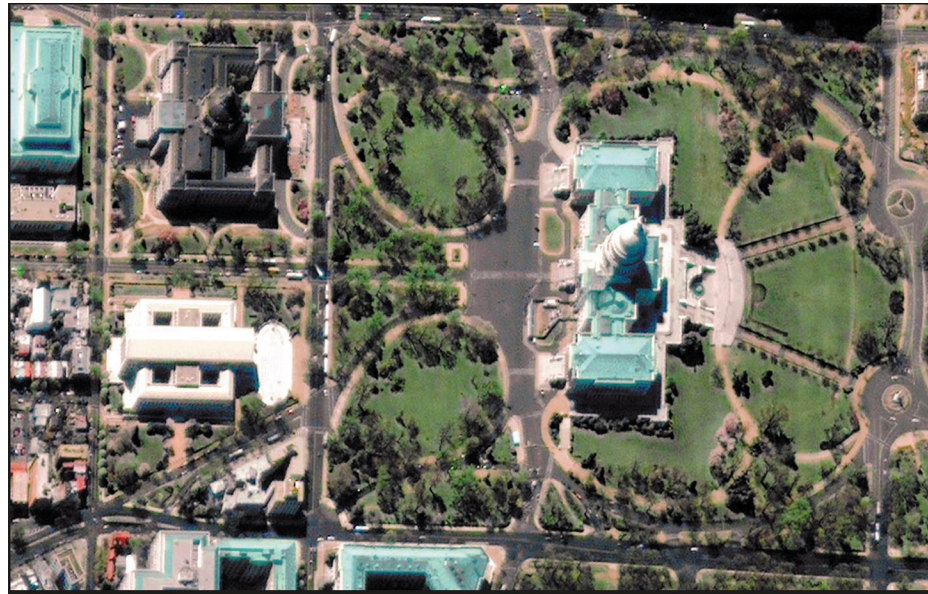
One-meter pan-sharpened color image of the U.S. Capitol, collected by Space Imaging's Ikonos satellite. This image demonstrates current, first-generation commercial space imagery capability.
