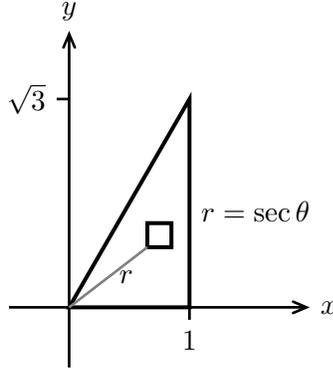
The polar moment of inertia is the moment of inertia around the origin (that is, the  $z$ -axis). The figure shows the triangle and a small square piece within  $R$ . If the piece has area  $dA$  then its polar moment of inertia is  $dI = r^2 \delta dA$ . Summing the contributions of all such pieces and using  $\delta = 1$ ,  $dA = r dr d\theta$ , we get the total moment of inertia is
