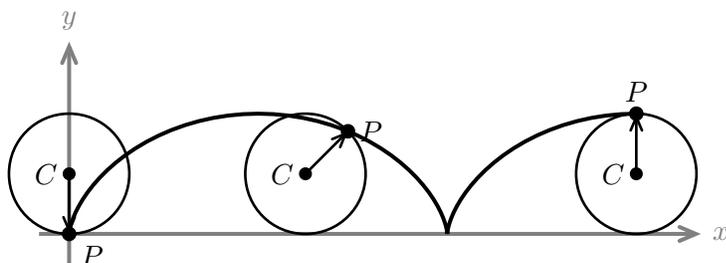
The natural parameter to use is the angle  $\theta$  that the wheel has turned. We'll use vector methods to find the position vector for  $P$  as a function of  $\theta$ .
