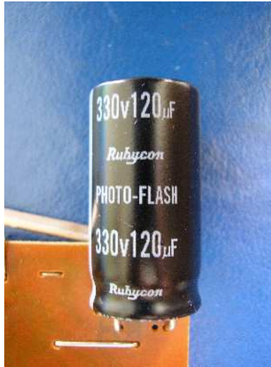
Figure 5.2.4: Electrolytic capacitor of a single use flash camera
